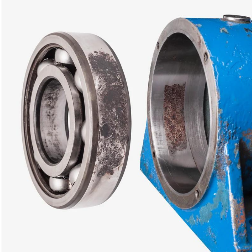
FIGURE 1.4 – Effet fretting corrosion
